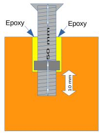
Insert screws with nut into epoxy filling; ensure to insert down into screw size hole for correct positioning.
